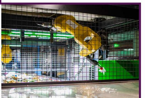
database of 2.5 million items – the innovation delivers higher granularity, speed, and affordability. Recycleye has also redesigned its robotic gripping function - the GRIP-R - to effectively handle films and flexible packaging and blockages.
